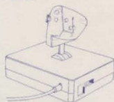
WCS - Weapons Control System - throttle + more. Held in left hand.
