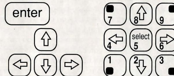
Numbers 1, 3, 7, and 9 take the cursor directly to the corners of the display; use the even-numbered keys for finer navigation.
