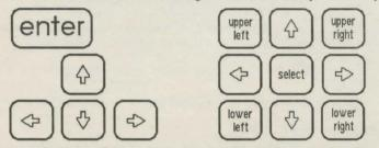
Numbers 1, 3, 7, and 9 take the cursor directly to the corners of the display; use the even-numbered keys for finer navigation.
