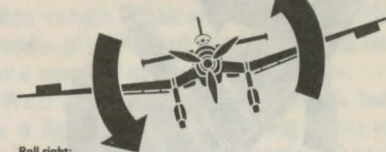
Roll right: push control column right
