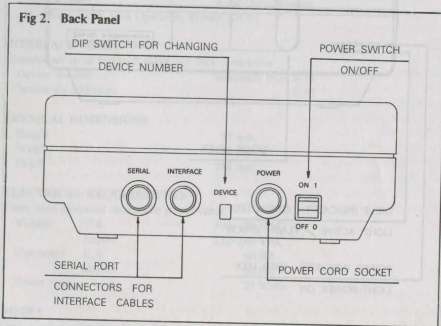
After plugging the power supply into the disk drive and a suitable outlet, find the black cable that goes from the disk drive to the computer. It is called a serial bus cable to describe the way the computer, and other accessories communicate with each other through its wires. It has an identical 6-pin DIN connector at each end, which like the power connector can only go in one way—with the dimple in the side of the plug facing up.
